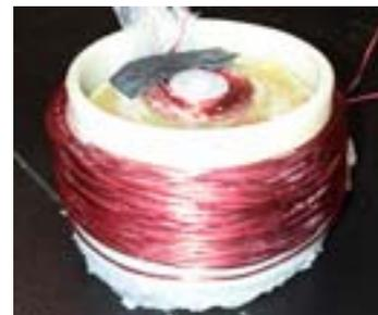
Fig 1: Transmit coil and one planar receive coil (the second receive coil is mounted on the bottom face of the transmit coil.).
