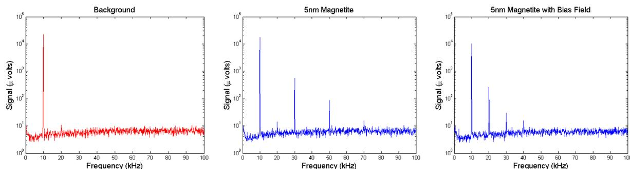
Fig 2: The harmonic signal from 5nm magnetite particles without a DC bias field (middle) and with a 0.2T DC bias field (right). The 12mT, 10kHz drive field contaminated the fundamental signal from the particles, and is shown as a background signal (left). The data was acquired without averaging using an Agilent CXA N9000A Signal Analyzer (resolution bandwidth = 56Hz).
