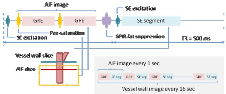
Fig. 1: Pulse sequence diagram of black-blood SHILO showing two TR intervals comprising one AIF image and one SE segment. Grey insert shows repetition of TRs for one SE vessel-wall image, which is then repeated for DCE imaging.
