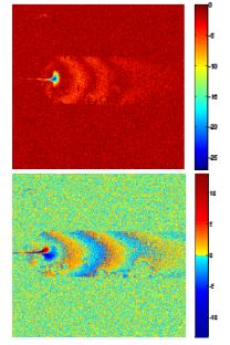
Fig 2 Real (top) and imaginary (bottom) part reconstruction of GRE image at 20 ml/h flow rate. Signal is normalized to the noise standard deviation calculated from 2 signal-free ROIs. One the real part one could see that DNP provide a negative enhancement relative to the thermal polarization. The laminar flow zone in the cell profile (parabolic phase variation) and jetflow zone near capillary inlet can be clearly distinguished.
