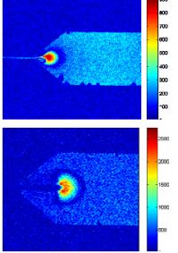
Fig 1a: Single shot SGRE image at 30ml/h flow. Sequence parameters: TR/TE=100/10ms Voxel size= 0.1x0.1x0.4mm. One can clearly observe the jet of hyperpolarized, thus hyperintense sample into the cell filled with thermally polarized sample.
