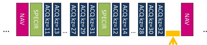
Fig. 1 Schematic description of navigated LAVA with a 20ms wait before navigator sequence (arrow). Image data acquisition does not start with kz of 1 due to partial kz acquisition scheme. Data are acquired in an interleaving way in the z direction.
