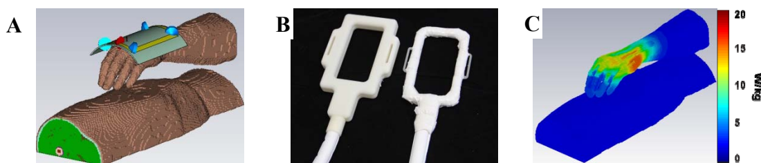
Fig. 1: A) Conductor layout of the 1 channel flexible Tx/Rx RF coil, B) Coil configurations left) flexible geometry right) rigid geometry C) SAR distribution over the voxel model's hand.
