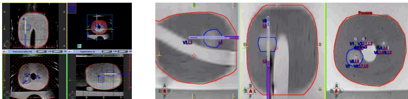
Fig. 2: Left: planning of biopsies in iso-echoic, MRI-only visible lesions in a CIRS 066 phantom; right: post-interventional MRI matched with the intra-interventional contours and registered biopsy trajectories.
