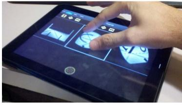
Figure 1: Real time MRI application running on tablet architecture. The scanner is controlled with touch and multi-touch gestures, on screen buttons, and physical keys such as the volume up/down keys for geometry control.
