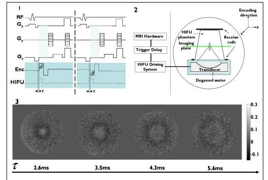
Figure 1: The MRI pulse sequence with displacement encoding gradients is shown on top left; Figure 2: The MR-ARFI system setup; Figure 3: The phase difference images at different  $\tau$  demonstrate the propagation of the displacement wave in the medium.
