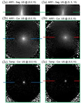
**Figure 2** (a) Sagittal slice through peak of 3D ARFI map when US fired at (0,0,15) (b) coronal slice through peak ARFI signal, ARFI signal along blue line plotted in figure 4a, (c) coronal slice of 3D temperature map; same slice location as (2b), temperatures along blue line plotted in figure 4b.
