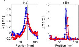
**Figure 4** (a) Blue: 3D ARFI signal along blue line in fig. 2b, US @ (0,0,15). Red: 3D ARFI signal along red line in fig. 3b, US @ (5,5,15). (b) Blue: 3D temperatures along blue line in fig. 2c, US @ (0,0,15). Red: 3D temperatures along red line in fig. 3c, US @ (5,5,15).
