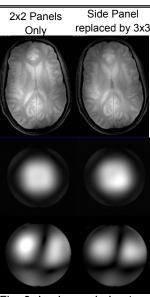
Fig. 3: In-vivo and phantom GRE images for the test configurations of the modular head coil.
