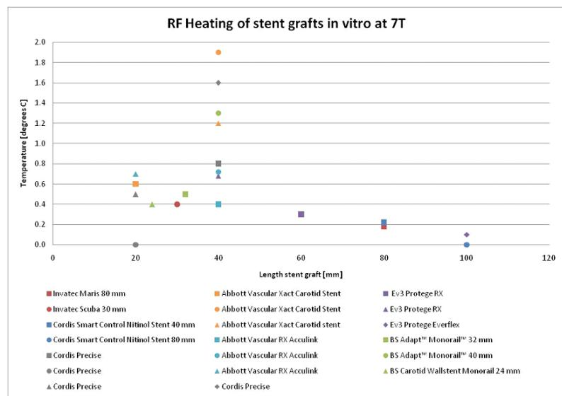
Figure 2: Temperature increases measured next to stents in phantoms while administering power which results in three times the federal SAR limit.
