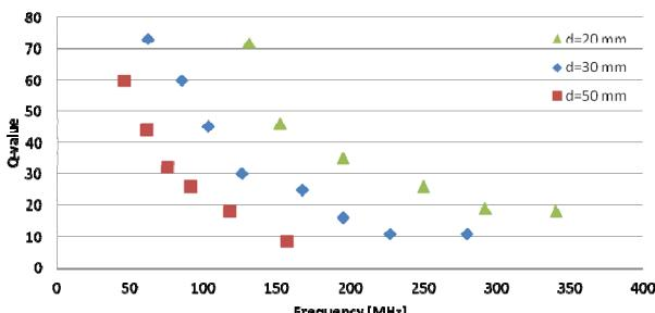
Figure 1: Quality factor of single loop coils resonating at frequencies ranging from 50 to 350MHz.
