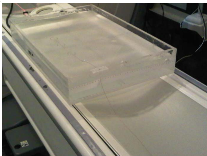
Figure 1: Photograph of experiment setup for the first experiment. The wire can be seen lying on the table in the bottom portion of the image. The PAA phantom lying on the MR table is seen in the upper portion of the picture.
