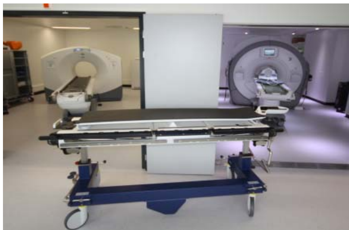
↑ Fig. 1: Patient transfer shuttle with special transfer-board on top in front of the PET/CT-system (GE Discovery 690) in the room on the left and the 3T-MR (GE Discovery 750) in the adjacent room to the right. The special transfer board allows for surface coil placement/removal between the exams even underneath the patient without patient repositioning.
