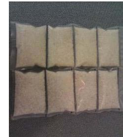
Fig. 1. HDC-pad with 50 mm sections to increase flexibility
