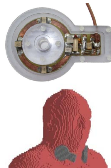
Fig.1: Top: Segmented loop coil for DC-CASL at 9.4 T. Bottom: positioning of coils on HUGO model.
