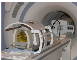
Figure 4: Imaging set up with oil phantom and paddles loaded in head holder, all inside TX coil.
