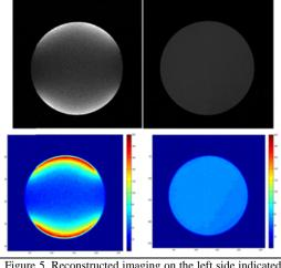
Figure 5. Reconstructed imaging on the left side indicated high SNR on the top-bottom configuration for cardiac imaging. The bottom SNR maps display 10 channel arrays combines higher SNR than volume coil reference imaging on the edge of phantom.
