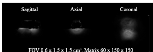
Fig. 2. A 3D FLASH image of the 1% agarose gel obtained by the parametric resonator with 100 \mu\text{m} isotropic resolution.
