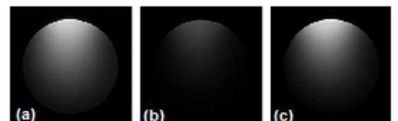
Fig. 4. Images acquired using a single element coil. (a) Unshielded; (b) Shielded without dielectric; (c) Shielded with dielectric.
