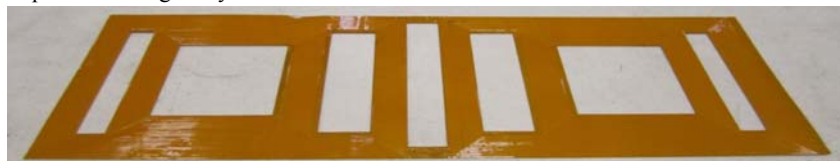
Figure 4. One of the Kapton circuit boards is shown that is impregnated into a widebore gradient coil to evaluate the image quality.
