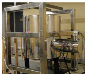
Fig.3 Magnet and aluminium frame for mounting the gradient coil.
