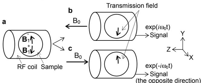
Fig. 1. A schematic of the rotating object method. The case of the inverted  $B_0$  is shown; the original (b) and the inverted (c) configurations.
