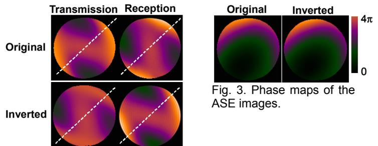
Fig. 2. Maps of transmission and reception fields of a saline phantom. The axis which passes through the feeding port in the RF coil are shown as the white broken lines.
