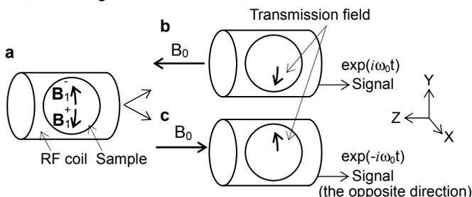
Fig. 1. A schematic of the rotating object method. The case of the inverted  $B_0$  is shown; the original (b) and the inverted (c) configurations.
