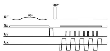
**Fig. 1** VAT-EPI sequence. Compared to standard EPI, there is an additional slice-axis gradient (shaded) applied during the entire readout period and the RF excitation pulse is elongated to reduce k-space modulation during the EPI readout.
