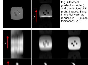
**Fig. 3** Coronal VAT-EPI images (top row) and corresponding slice profiles (bottom row) for excitation RF pulse widths, from left to right, 4.3, 18.7, 43.6 ms. For the slice profiles, a coronal slice-selective excitation was followed by a sagittal projection acquisition.
