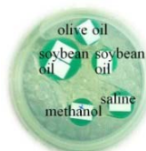
Fig 3. A custom-made phantom used for the experiment
