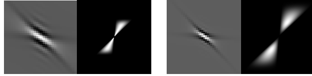
Figure 1: Image of one mid-scale shearlet and its spectral support for the low redundancy shearlet transform (left) and the proposed smooth radial shearlet transform (right)
