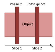
**Figure 1:** Phase difference  $\Delta \phi$  between simultaneously excited slices is used to improve image reconstruction.
