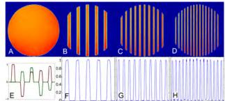
Figure 2: Images of a silicone oil phantom excited using a non-selective excitation pulse (A), and multislice excitation pulses with N=5,10,15 (B-D). Magnitude profiles are shown in F-H, and E shows separate real and imaginary components of the 5 slice excitation, with calculated profiles in black.
