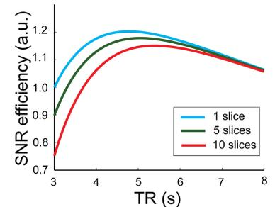
Figure 1. Calculated SNR efficiency as a function of TR for different number of slices.
