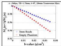
Figure 3: Ratio vs b-value for each phantom at  $\Delta=360\mu s$ .
