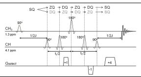
Figure 1; refocused double quantum selection sequence. The lactate signal is converted to a double quantum state where it is twice as sensitive to dephasing gradients. The overlapping (single quantum) lipid signal experiences asymmetric gradients and shows a reduced signal intensity, dependent on the effective spoiling area. The first excitation pulse was made slice selective to generate signal from a single slice.
