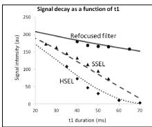
Figure 2; lactate signal with a SSEL, HSEL or refocused double quantum filter. The refocused filter shows no additional signal loss (apart from T2 decay)
