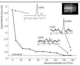
Figure 3; measurements were performed with the double-quantum read pulse turned off, and with increasing dephasing strength. After the lipid residual signal was reduced to below the noise level, the double-quantum read pulse was turned back on, and a clear lactate signal was detected.
