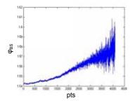
**Figure 2:** Bloch-Siegert phase shift  $\phi_{BS}$ . To calculate predicted optimal gain  $TG_{predicted}$  the mean value of first 1024 points is used.
