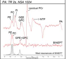
Figure 3: BINEPT and PA MR spectra of the breast of a healthy volunteer at 7Tesla. The PCr, and NTP signals originate mainly from the muscle tissue and are out of phase due to a frequency offset in the muscle compared to the breast. The glandular tissue volume was ~150cm³. BINEPT: TR 2.5s, NSA 150. PA: TR 1.5s, NSA 249
