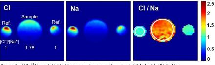
Figure 1: <sup>35</sup>Cl, <sup>23</sup>Na and divided image of phantoms. Sample vial filled with 1% NaCl and 1% KCl yielding an ion concentration ratio [Cl]/[Na<sup>+</sup>] of 1.78:1.
