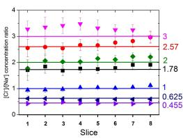
Figure 2: Known CI/Na<sup>+</sup> concentration ratio of the samples (solid lines) and measured concentration ratios derived from ROIs within the concentration ratio map (compare Fig.1).
