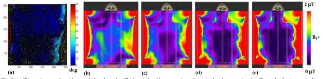
Fig. 1. (a) Flip angle map of a mid-coronal slice through a Thiel-embalmed human cadaver. Intensity levels proportional to flip angle; (b-e) numerical computed B1+ maps for male HBM for electrical conductivities of (b) 1 S/m, (c) 2.6 S/m, (d) 5.8 S/m, and (e) 10.6 S/m
