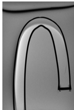
Phantom tests with a NaCl-filled model (left) of an aortic arch. A conventional steel guidewire (middle) and the devolped CFRP-guidewire prototype (right) were advanced separately through the arch. The steel guidewire provokes strong artefacts whereas the newly developed guidewire is nearly artefact free. Both wires were investigated under identical parameters.
