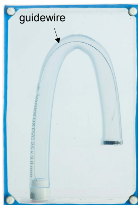
Phantom tests with a NaCl-filled model (left) of an aortic arch. A conventional steel guidewire (middle) and the devolped CFRP-guidewire prototype (right) were advanced separately through the arch. The steel guidewire provokes strong artefacts whereas the newly developed guidewire is nearly artefact free. Both wires were investigated under identical parameters.
