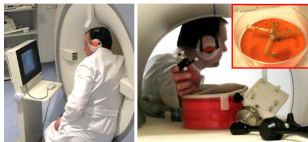
Fig. 2: Proof of concept for automatic scan-plane prescription. Left: The procedure is performed from the scanner's back end and guided by near real-time MR images along or perpendicular the instrument that are displayed on the in-room console. Right: View from the opposite end with tracker and reference board inside the bore. Inset illustrates layout of the phantom with targets (peas, mean Ø 8.5 mm) and vessel model embedded (here: partially) in opaque glaze.
