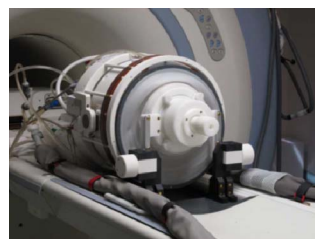
Fig.1: The phas array transducer setup with a dedicated 8-channel phas array receive coil, a gel phantom mounted inside the hemisphere and water lines for circulating water through the transducer.
