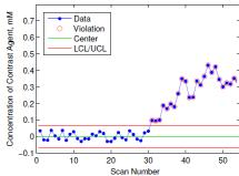
Figure 1: Example of the control chart rules applied to a contrast agent curve. This data set indicates a BAT at scan 30.
