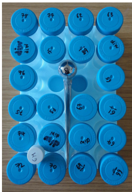
Figure 1: Plan view of phantom containing plastic vials of \text{CrCl}_3 solutions in a plastic rack with a metal hip at the centre of the phantom.
