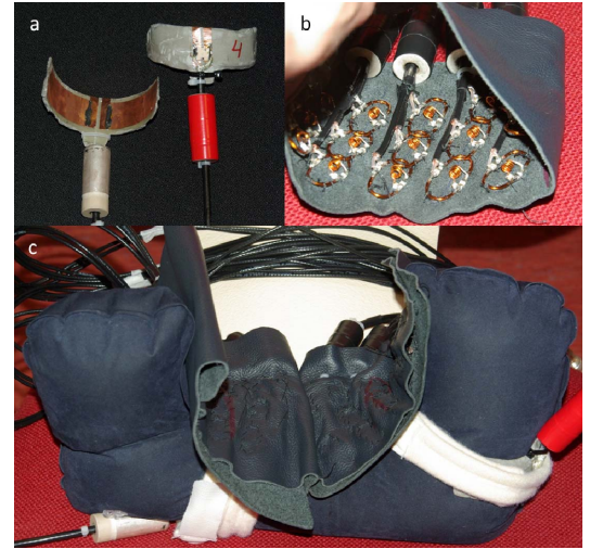
Figure 1: Coil setup: two radiative transmit antennas(a) were attached to the outside of a neck pillow filled with D 2 O (c); a 30-channel receive coil (b) was placed close to the neck on the inside (c) of the neck pillow.
