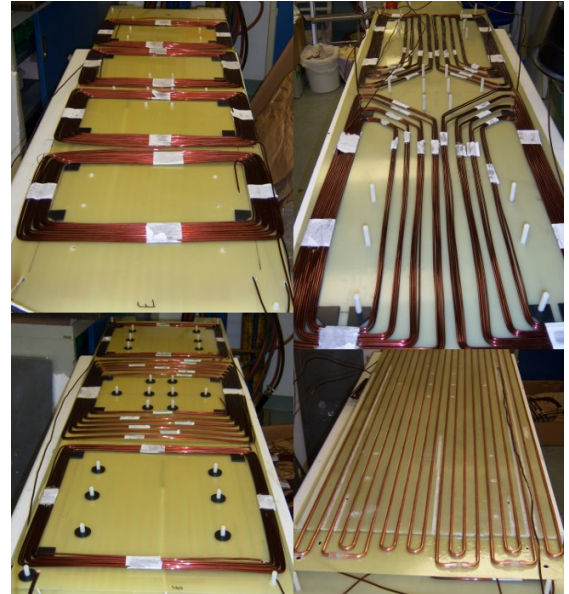
Fig. 1: Coil elements for each channel and one layer of water cooling tubes with grooves for temperature sensors and connectors.
