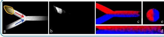
Fig 2: Flow observation at a "Y"-shaped tube junction. (a) conventional TOF imaging with marked label volume. (b) excitation of the labeling volume with saturation pulse. (c) longitudinal section (d) with zoomed boundary layer and (e) transversal section through superimposed difference datasets
