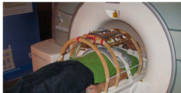
Fig. 1: UWB setup in front of the 3T scanner.
