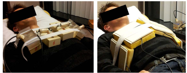
Figure 1: Positioning of array elements on volunteer a) radiative antennas b) loop coils
