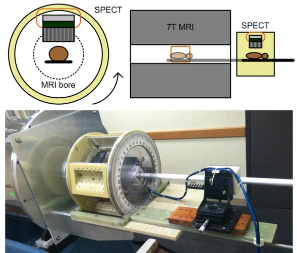
Fig. 1. Axial view, side view, and photo of the integrated 7T MRI and SPECT systems
