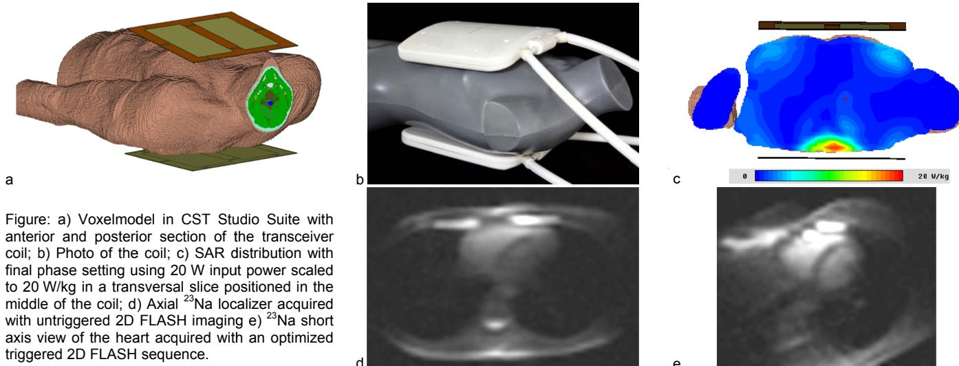
Figure: a) Voxelmodel in CST Studio Suite with anterior and posterior section of the transceiver coil; b) Photo of the coil; c) SAR distribution with final phase setting using 20 W input power scaled to 20 W/kg in a transversal slice positioned in the middle of the coil; d) Axial  $^{23}\text{Na}$  localizer acquired with untriggered 2D FLASH imaging e)  $^{23}\text{Na}$  short axis view of the heart acquired with an optimized triggered 2D FLASH sequence.
