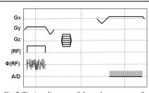
Fig.2 Timing diagram of the pulse sequence for the proposed 3-D hybrid encoding scheme.
