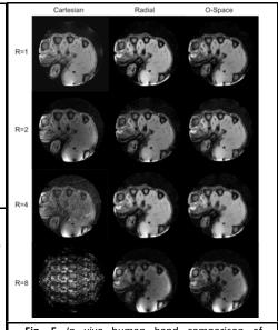
**Fig. 5** *In vivo* human hand comparison of Cartesian, radial, and O-Space 256×256 images using equivalent amounts of under-sampled data. R=1 corresponds to 256 readouts. A  $B_2$  inhomogeneity artifact is visible at the bottom of the hand. (FOV=10 cm)
