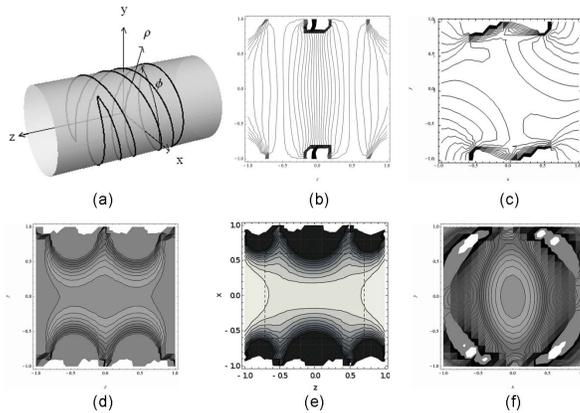
**Fig. 1:**  $G_z$  phase-gradient coil for horizontal  $B_0$ . (a) coil, (b) phase plot in sagittal plane, (c) phase plot in transverse plane, (d) magnitude plot in sagittal plane, (e) magnitude plot in coronal plane, (f) magnitude plot in axial plane.
