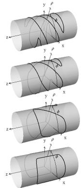
**Fig. 3:**  $G_z$  coils for  $s=\pi$  (top) to  $s=0$  (bottom).
