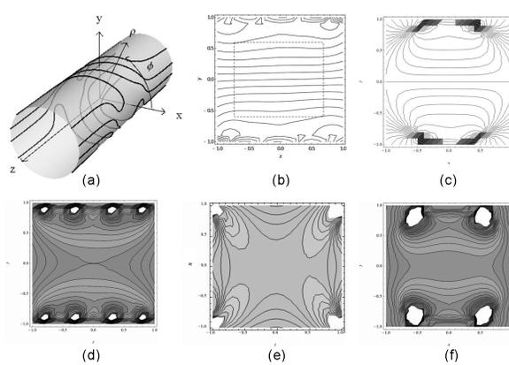
**Fig. 2:**  $G_y$  phase-gradient coil for vertical  $B_0$ . (a) coil, (b) phase plot in sagittal plane, (c) phase plot in axial plane, (d) magnitude plot in sagittal plane, (e) magnitude plot in coronal plane (f) magnitude plot in axial plane.
