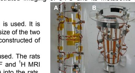
Fig. 1. Developed RF coils. **A:**  $^{19}\text{F}$  two-element phased-array coil; **B:**  $^{19}\text{F}/^1\text{H}$ -dual tuned linear birdcage coil.
